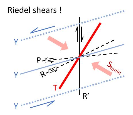
T – tensile fracture, azimuth 32° controlled by the stress field;
