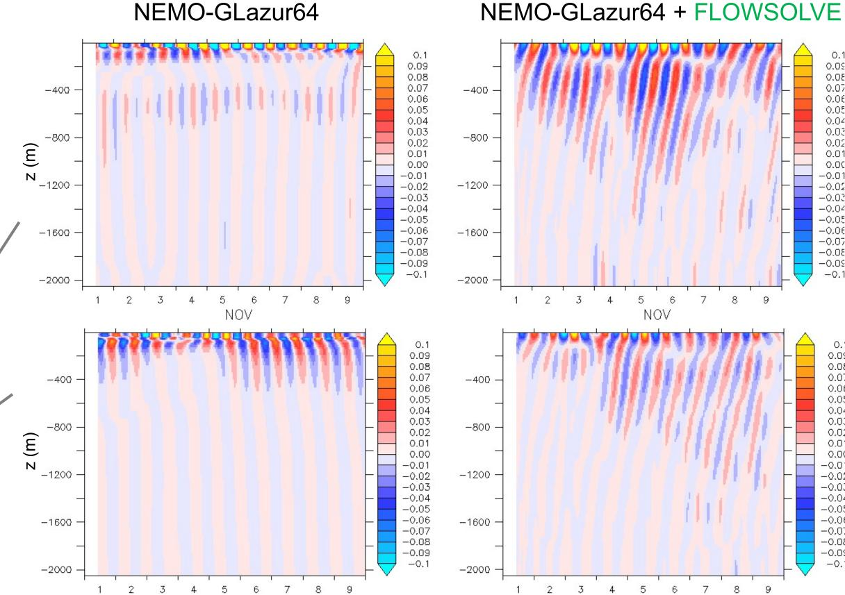
Hövmoller diagrams of high-passed zonal velocity (m s<sup>-1</sup>)
