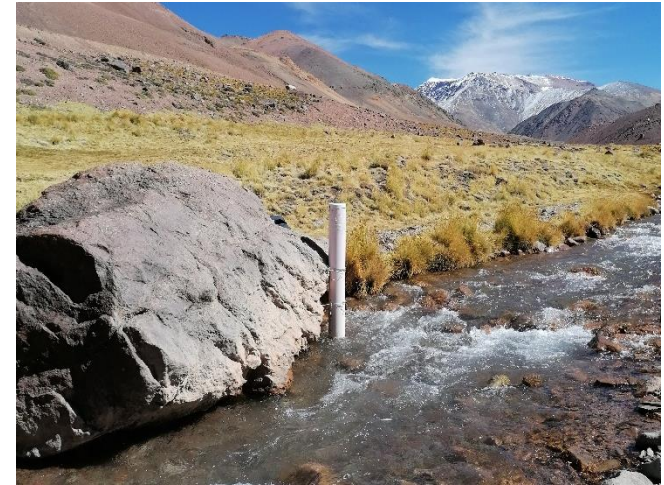
Figure 8: One of the six gauging stations continuously measuring discharge along the Agua Negra river
