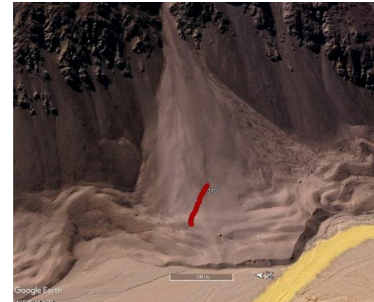
Figure 12: Vertical ERT profile measured in the lower part of a talus slope located at the lower limit of the upper Agua Negra catchment (around 4100 m asl). The electrical resistivity values ( > 35 \text{ kohm.m} ) are compatible with permafrost and its distribution is related to the base of the talus (the steepest part of the profile), as described by Lambiel and Pieracci, 2008. SRT was carried out at the same ERT location, and the data is currently processed.
