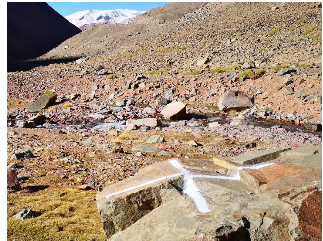
Figure 5: Example for ground control points used to georeference UAV-based DEMs
