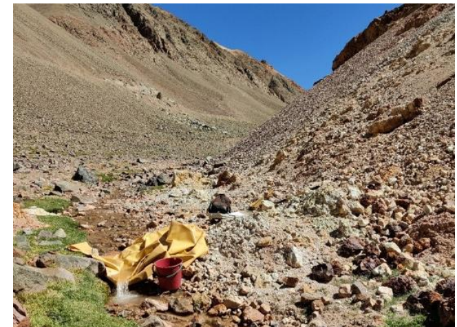
Figure 9: Repeated bucket measurements at Dos Lenguas rock glacier spring
