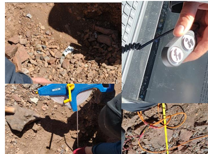
Figure 7: Setting and Installation of an iButton to record temperature at the midpoint of an ERT profile measured on a Talus slope
