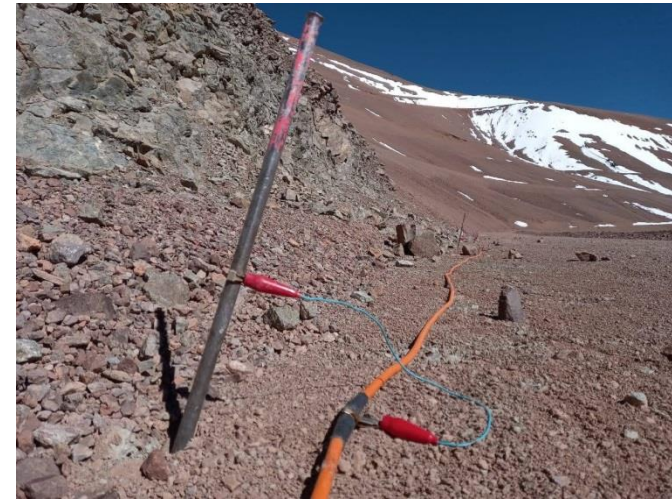
Figure 6: Longitudinal ERT profile measured on a blockslope in the upper Agua Negra catchment
