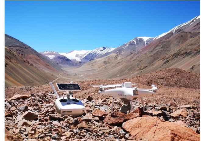
Figure 4: Phantom 4 RTK drone and controller used in the Agua Negra catchment.
