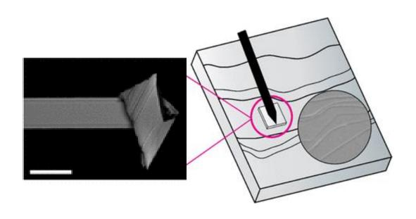
We used **Atomic Force Microscopy (AFM)** to study adhesion between two calcite surfaces
