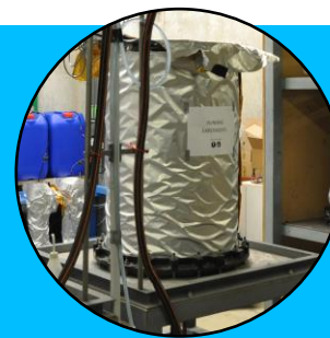
Lysimeter (variably saturated)
