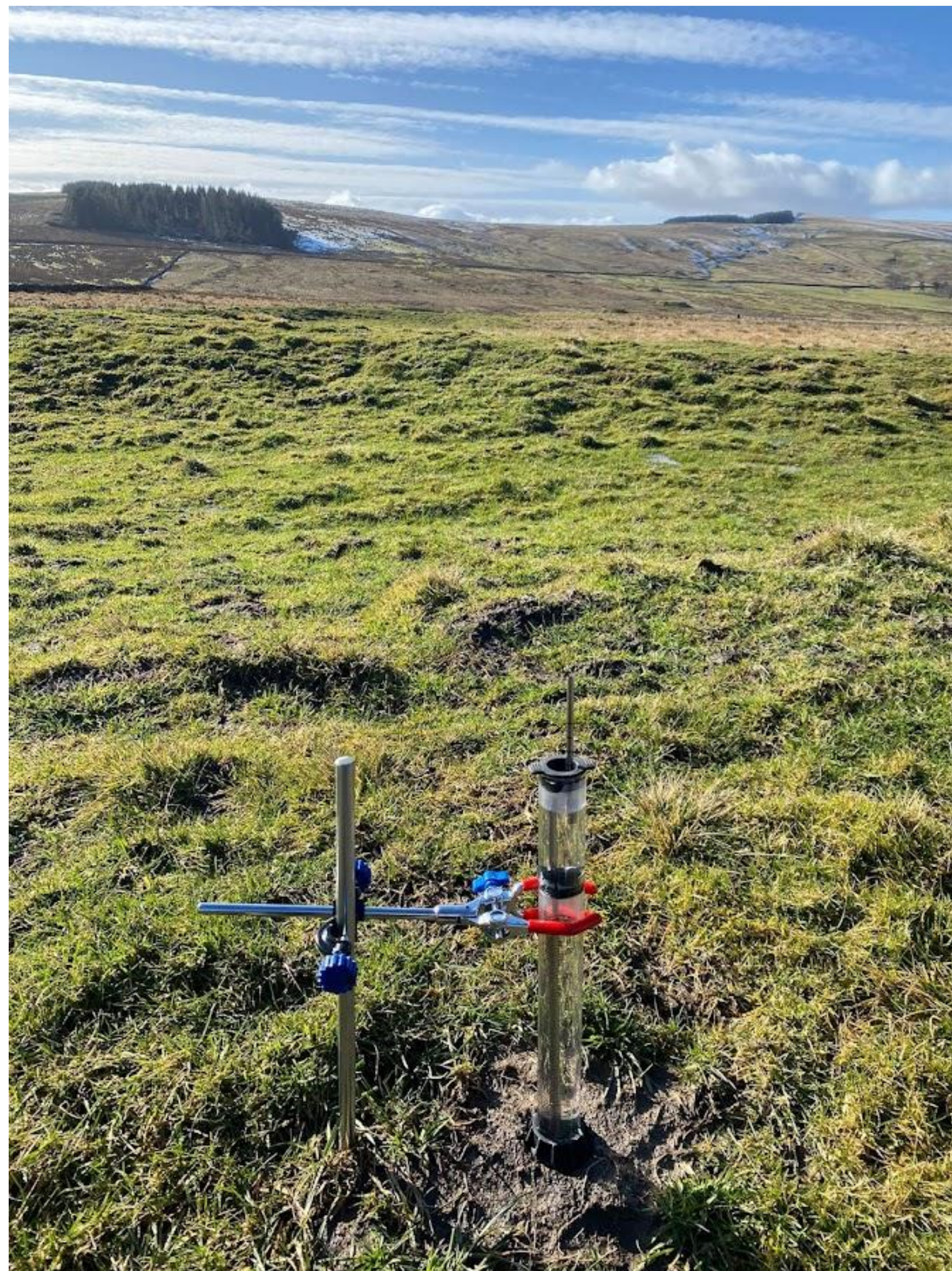
Figure 5. Installed mini-disk infiltrometer
