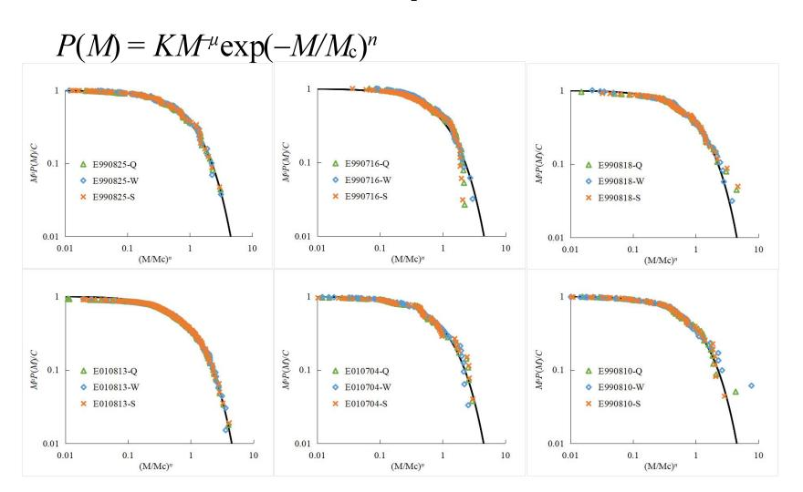
Both **simulated** sediment sequences and **real** events: single exponential curve
