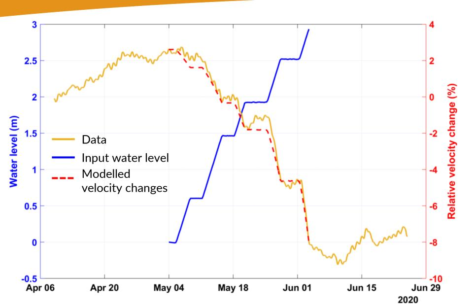
Model based on the increasing sensitivity of velocity changes to increasing water level
