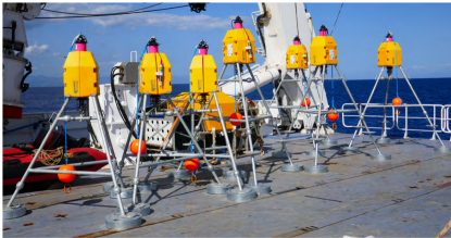
Geodetic stations deployed during cruise FOCUS-X1
