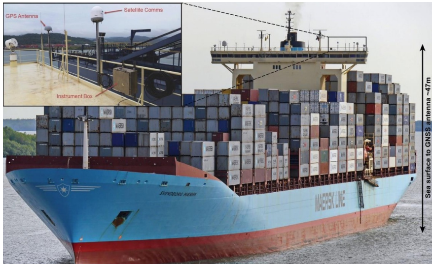
Figure: A installed Trimble NetR9 receiver GNSS receiver on the commercial ship [Foster, 2019]
