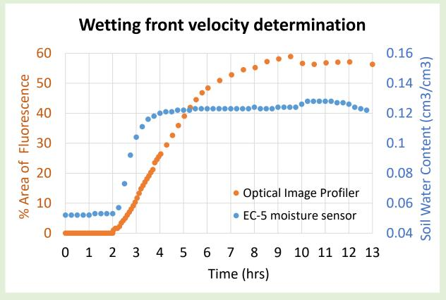
Detection of tracer at 122 & 130 minutes by OIP & EC-5 sensor respectively
