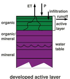
Part of the PWBM schematic from Rawlins et. al, (2013)
