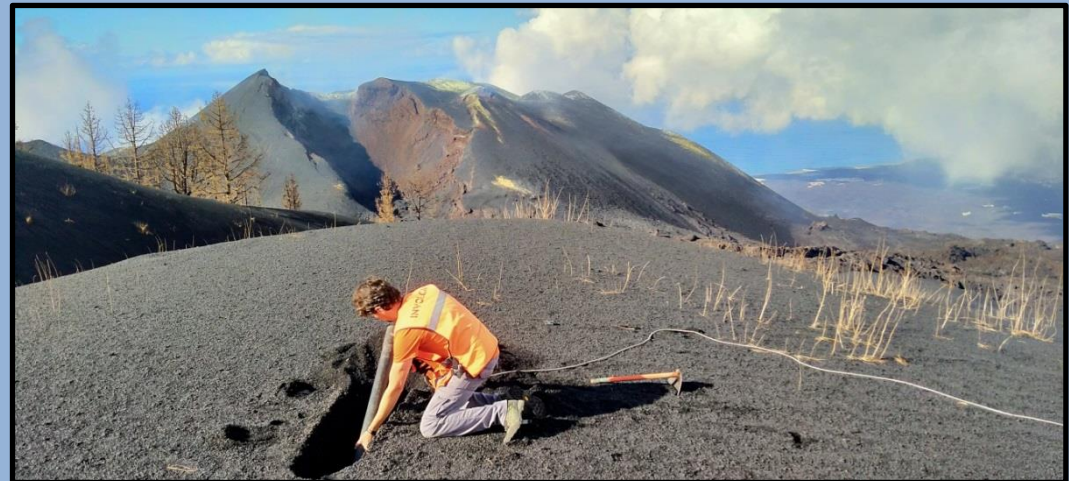
Installation of a magnetotelluric station
