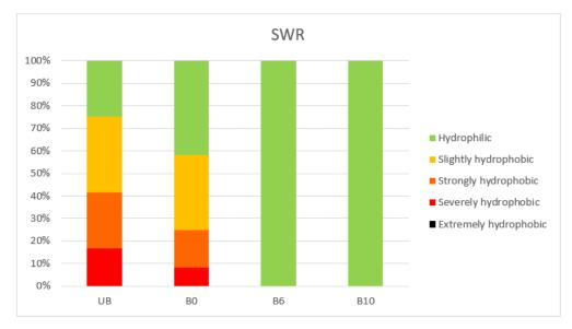
Occurrence (%) of Soil Water Repellency (SWR) according to the Water Drop Penetration Time (WDPT) test in the different sampling plots. SWR classes defined by Doerr (1998).
