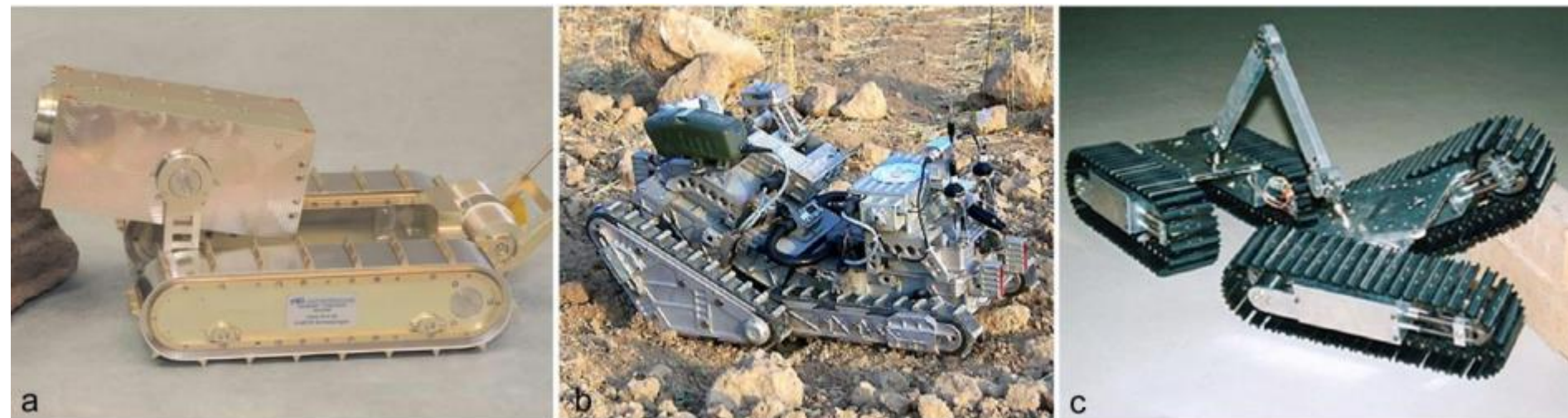
Tracked robots: Nanokhod (a, Klinker et al., 2007), Robhaz DT3 (b, Woosub et al., 2004) and Gunryu (c, Hirose et al., 1996).
