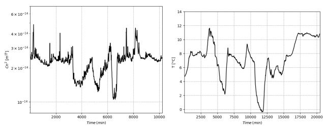
Measurements of  ${\cal C}_n^{\ 2}$  and T with a LAS MKI and a CNR4 respectively, in December 2019 and January 2020.
