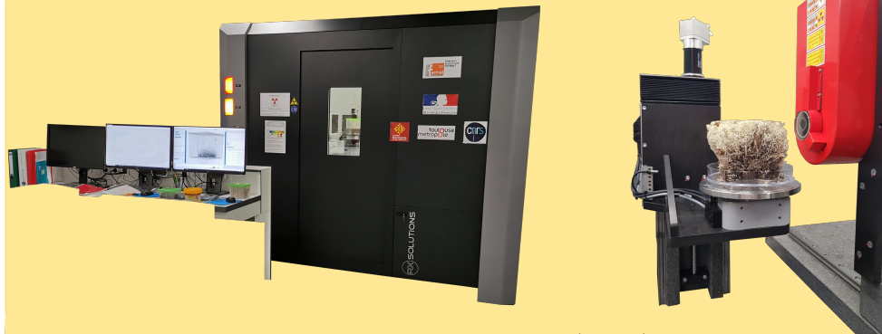
X-ray Computerized Tomography (X-CT), IMFT
