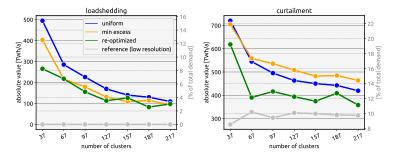
$\Rightarrow$  Load shedding in "min excess" similar to "re-optimized" results and 1-5% lower than in "uniform". (++)
