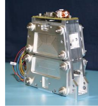
ISA accelerometer for the ESA BepiColombo mission
