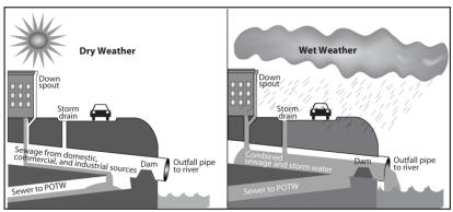
**Combined Sewer Overflows**determine the **discharge** of polluted water into water bodies when
