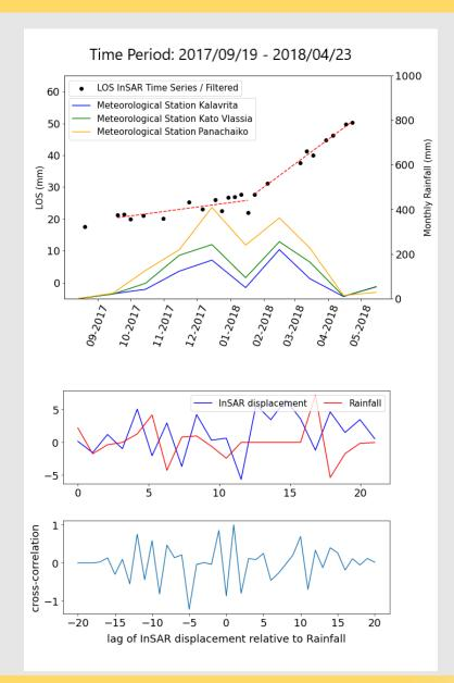
Two of the three time periods show an increase of displacement rate about 40%. The period September 2017-April 2018 shows an increase of the displacement rate about 550%. This result is accompanied by a large amount of total rainfall.
