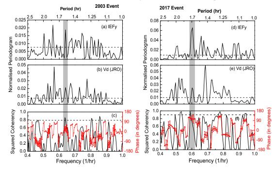
The DP2 type quasiperiodic fluctuations of 1.5-2 h in the vertical drift over Jicamarca are found to have causal connection with the similar fluctuations in IEFy.
