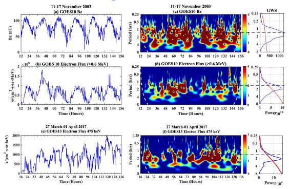
Quasi-periodic oscillations of 1.5–2 h are observed in the Z-component of the magnetic field for the 2003 event and electron fluxes at geosynchronous orbit for both the events.
