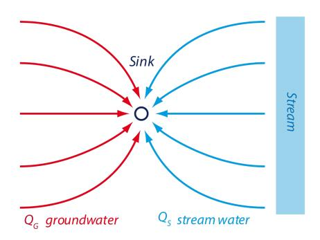
**super fast transport model** for : non-reactive advective transport with steady state flow
