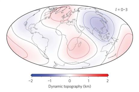
these models are already calculating the stress field of the flowing mantle! convective stress balances hydrostatic pressure at the surface
