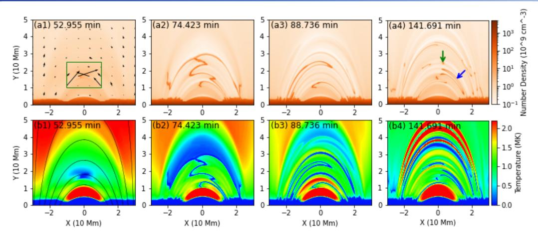
localized heating → evaporation → density increase, temperature first increases but then starts to reduce → thermal instability → condensations
