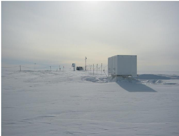
FIG. 1. The bistatic minisodar at Summit Station is in the foreground; shown are the two boxes that house the transmitting and receiving antenna systems. The meteorological tower, which held the 3D sonic anemometer that was implemented in this study, can be seen in the distance.
