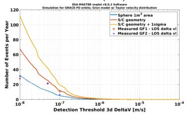
Measured data (crosses, circles) match the predictions from particle density models. Deviation at  $1\times 10^{-8}\,\mathrm{m\,s^{-1}}$  since MTE's can not be detected well in LRI data at these low  $\Delta v$  values.
