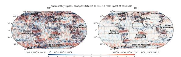
LRI and KBR show same signal (see e.g. Amazon watershed), but LRI has higher SNR / lower noise (especially over the oceans) Image Credit: [7]
