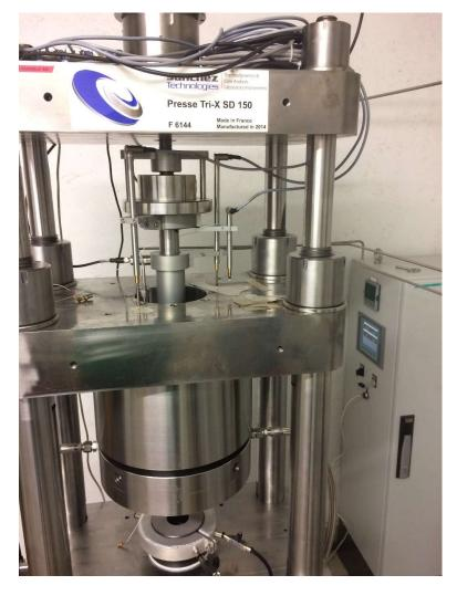
Griggs rig deformation experiments with Acoustic Emission (AE) recording
