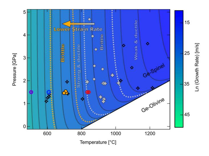
The transformational faulting temperature window previously described for strain rates of  $\sim 10^{-4} \text{ s}^{-1}$  is found here at lower temperatures for lower strain rates of  $\sim 10^{-5} \text{ s}^{-1}$ . This illustrates the control of both strain rate and transformation kinetics on faulting.
