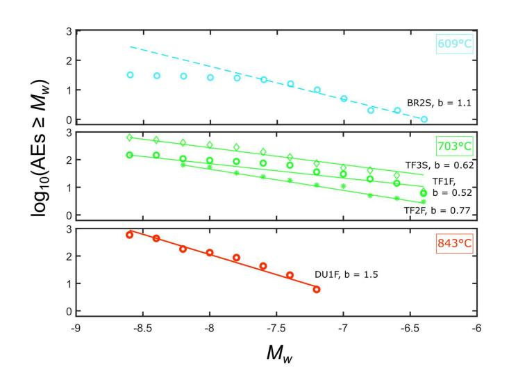
At 600°C, the *b*-value of 1 is consistent with standard brittle failure.
