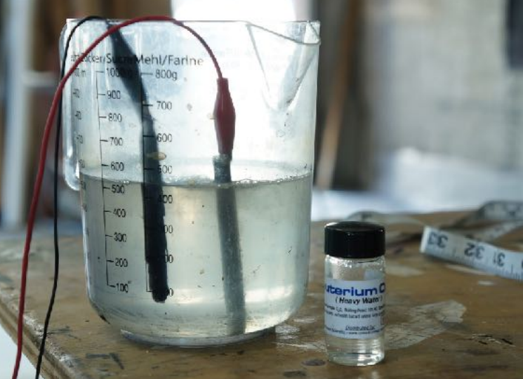
Enriching H 2 O with D 2 O via electrolysis
