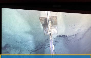
Rugged relief (scarp / cliff) → unburied cable (span)
