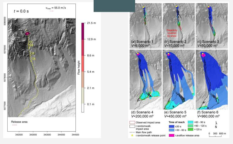
4) Forward simulations of scenarios of ice avalanches of different volumes with r.avaflow, resulting in estimates of travel time and flow pressure for each scenario.
