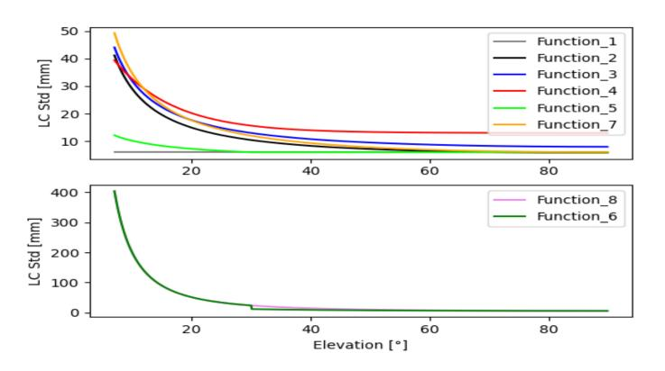
Standard deviations of carrier-phase of ionosphere-free linear combination with function of elevation angle for analyzed weighting functions.
