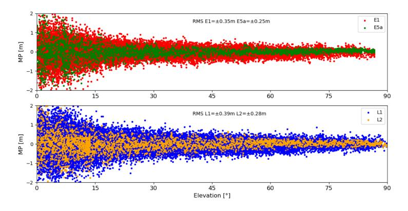
Multipath code combination (MP) for the E1 and E5a observations for the Galileo and L1 and L2 observations for the GPS for the MAS100ESP station for the 39 DoY with function of elevation angle.
