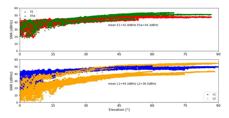
Signal to noise ratio (SNR) for the E1 and E5a observations for the Galileo and L1 and L2 obser-vations for the GPS for the MAS100ESP station for the 39 DoY with function of elevation angle.
