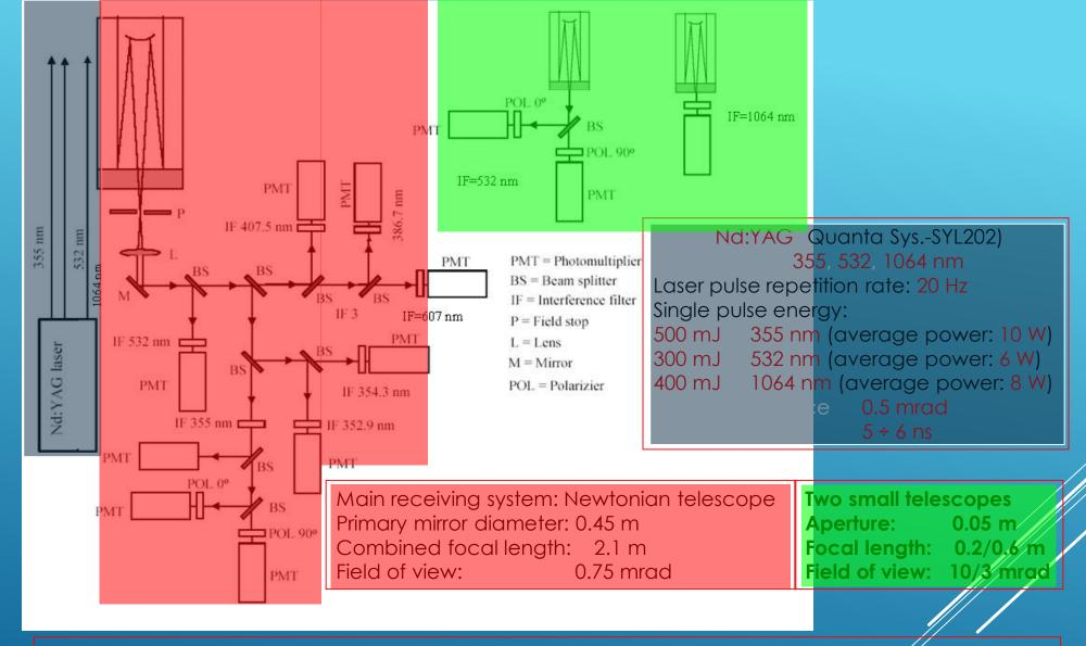
SPECTRAL SELECTION: based on Interference Filters
