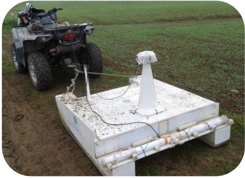
Soil mapping with EMI sensor (3 depths)
