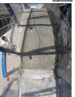
Simulation of uncovered soil that receive water from upstream snow melting water activity. Temperature of soil assumed to be in equilibrium to the air temperature (20°C).
