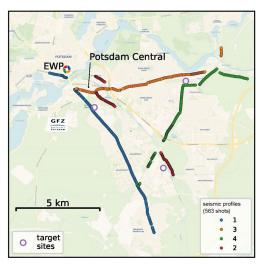
4530 sensor nodes along dark fibre 106 vibro points as active source
