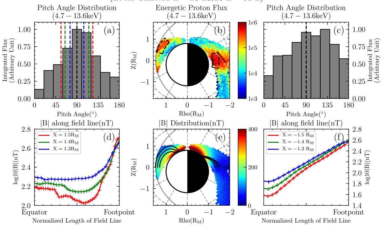
90 degree dominant pitch angle distributions and the off equator B field minimum on the dayside
