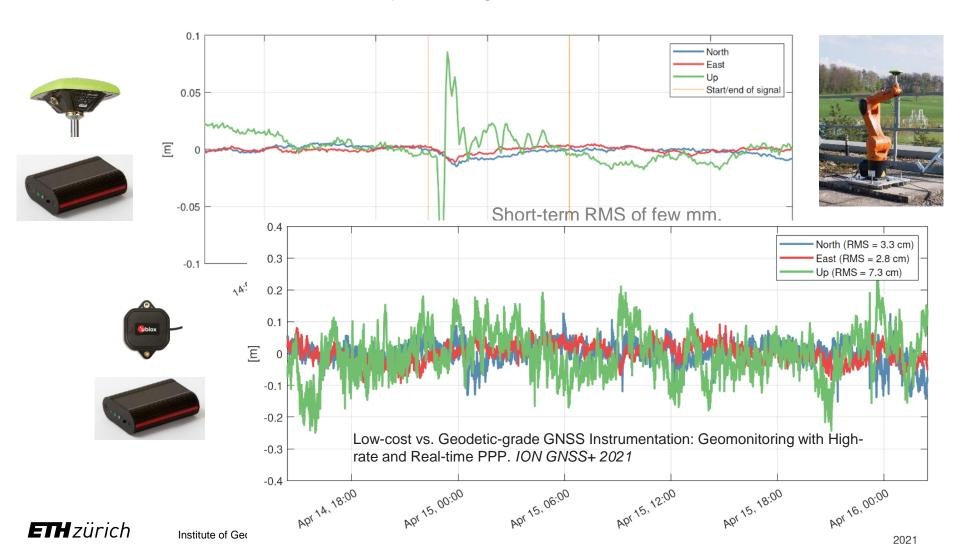
Experiment with robot, Real-time PPP, CNESdemonstrator software
