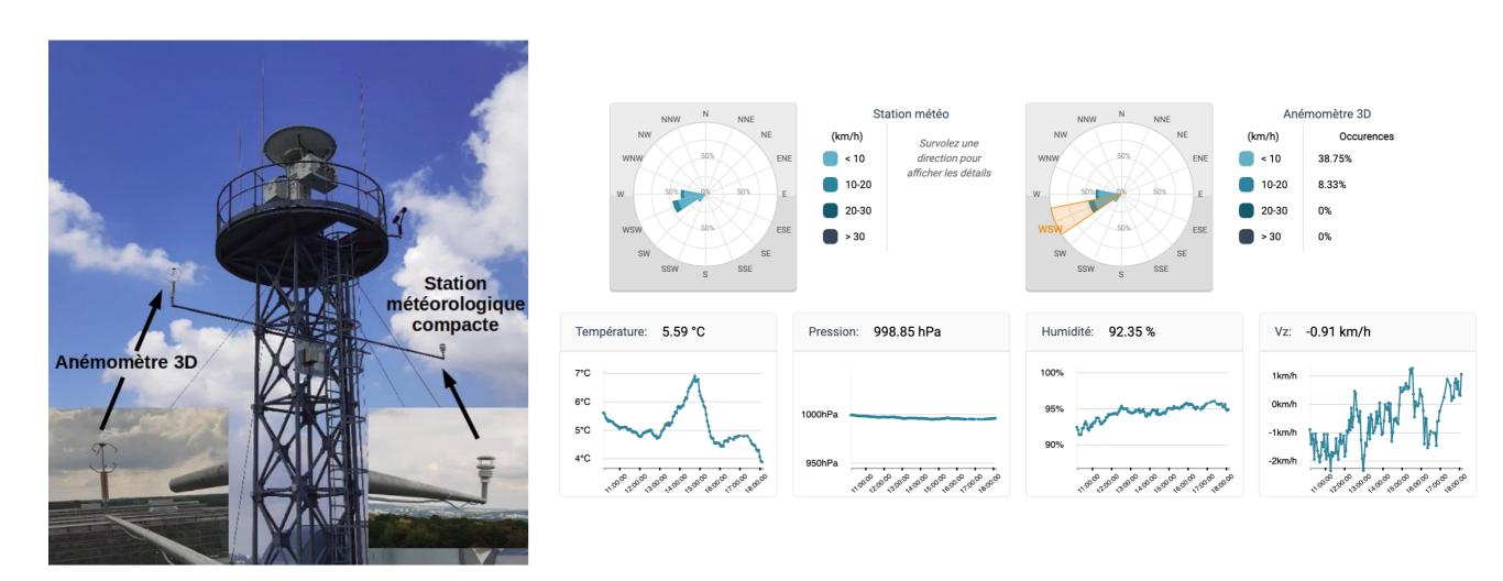
3D sonic anemometer and a meteorological station (ThiesCLIMA) provide information about the weather situation at the radar position such as 3D wind, temperature, pression and humidity.
