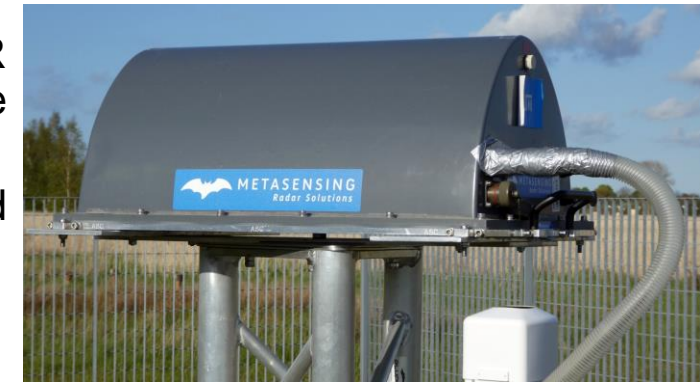
Electronic corner reflector in Łeba, Poland (LEBA) (photo by R. Zdunek)
