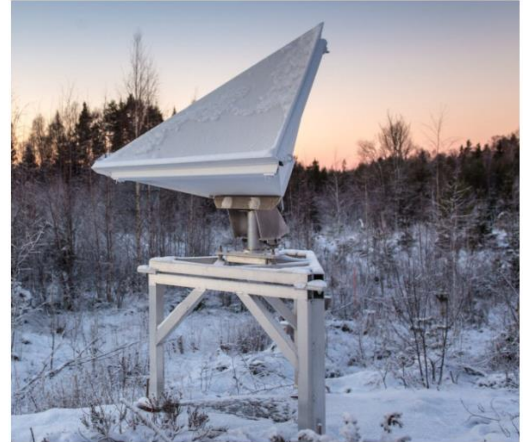
1.5 m corner reflector of Metsähovi station (Finland) (picture from Survey Protocol for Geometric SAR Sensor Analysis, 2018)
