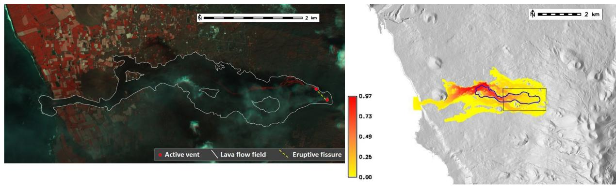
RGB composite (Band 4,2,1) of the Planetscope image acquired on 29 September 2021 at 11:25 GMT. The white contour delineates the lava flow field, the dashed yellow line the eruptive fissure, while red dots are the active vents.
