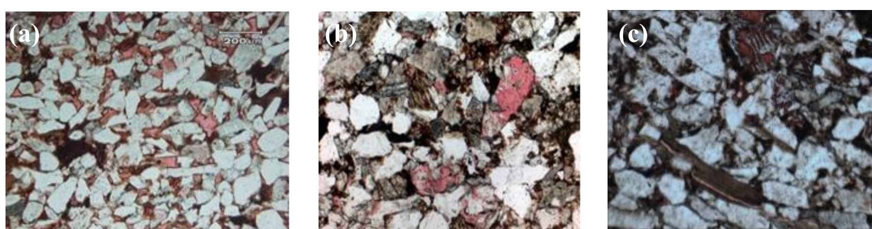
Figure 7. Chang 6 3 reservoir sandstone pore types in Huaqing area (a) B111, 2114.0 m, Intergranular pores; (b) B115, 2210.2m, Feldspar dissolved pore; (c) B123, 2092.1m, Muddy mica micro-cracks
