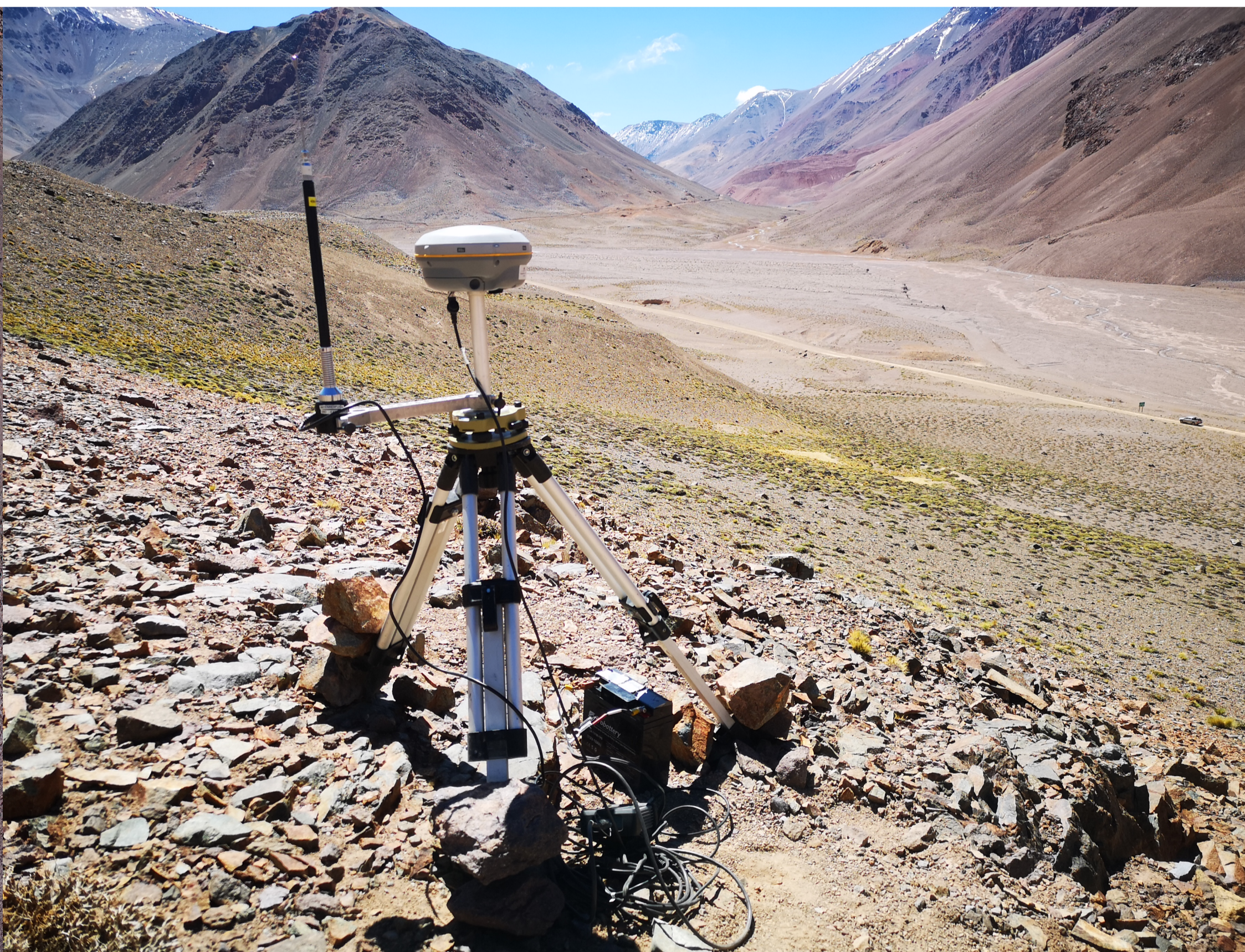
Figure 7: DGPS base as used during field campaigns 2022 and 2023. View towards Dos Lenguas (visible in the back). Own image, March 2022.
