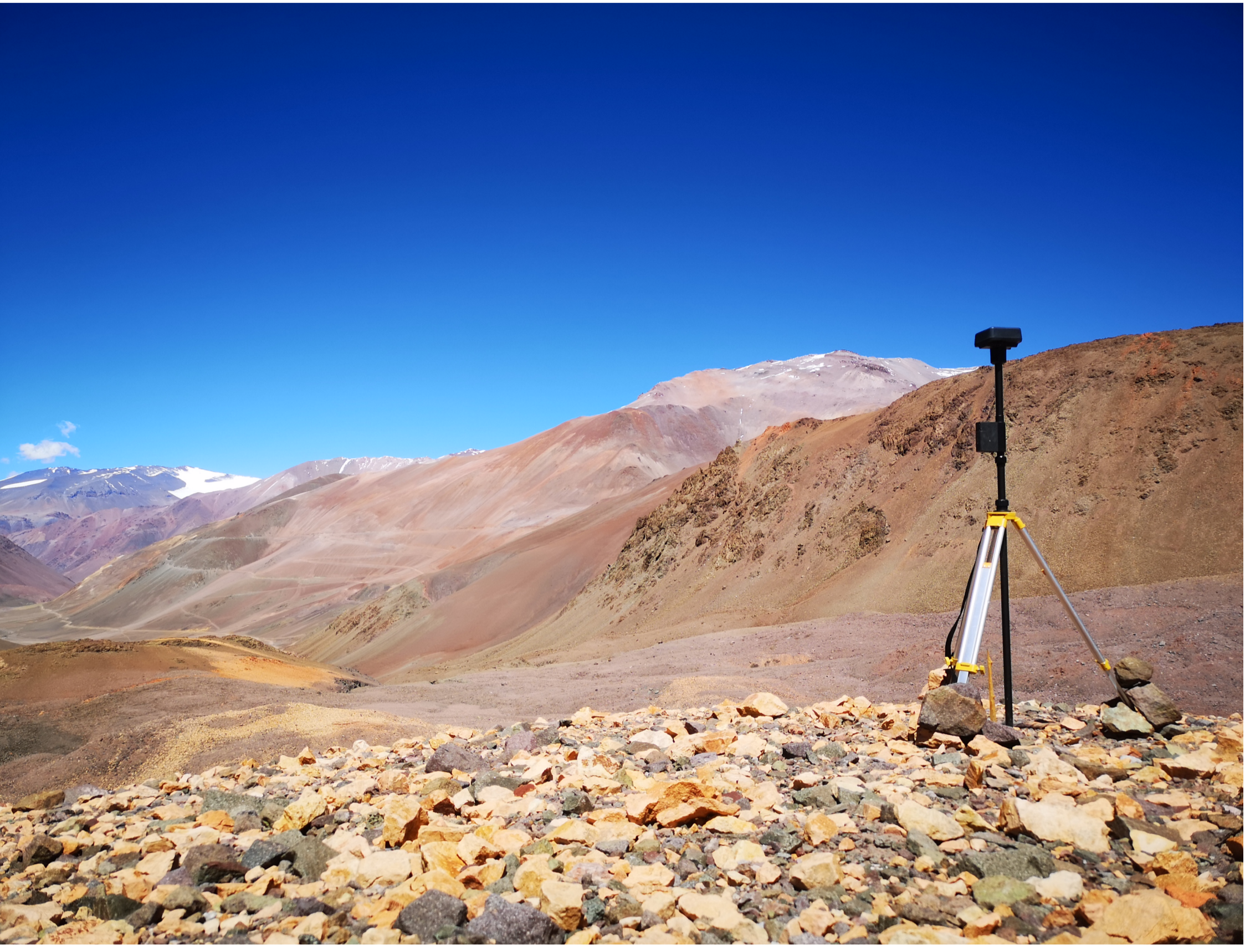
Figure 4: RTK equipment as used during field campaigns in 2022 and 2023. RTK base located in Agua Negra glacial forefield with southwards view along the valley. Majadita glacier is visible in the back. Own image, February 2022.
