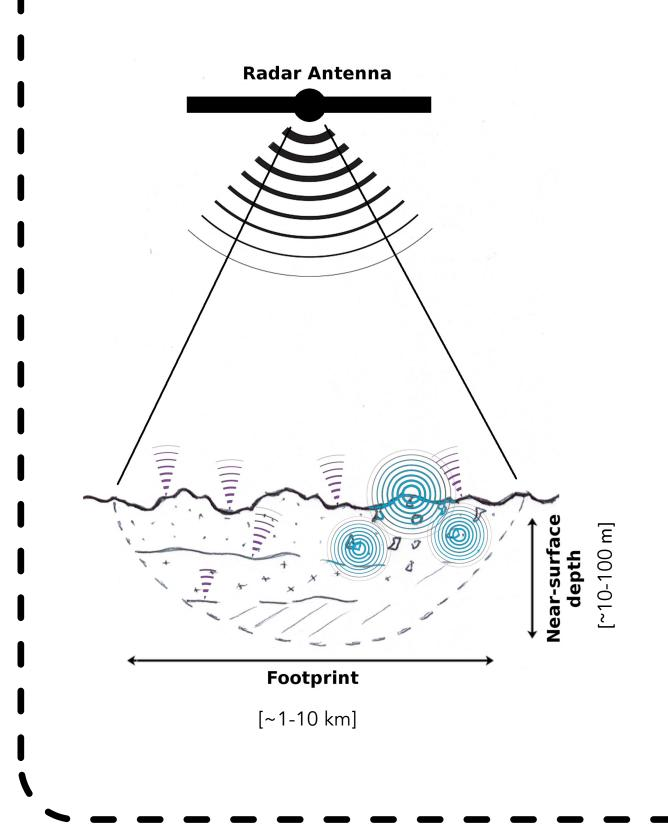
\*The near-surface depth is defined vertical as the resolution (i.e., skin depth) of each radar system.
