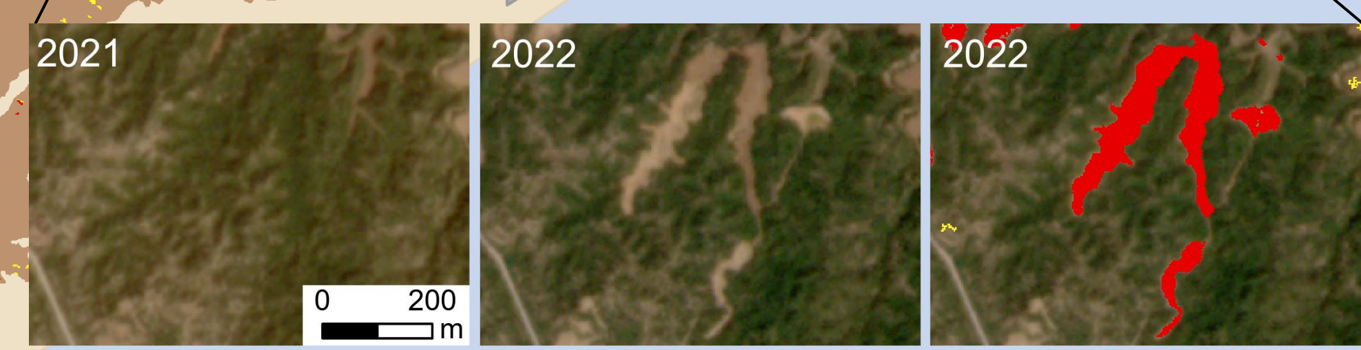
Figure 2: Area levelled in 2022 as detected by the algorithm. The levelling extent is accurately delineated.
