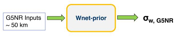
Trained by downsampling the high-resoltuion atmospheric simulation (G5NR)
