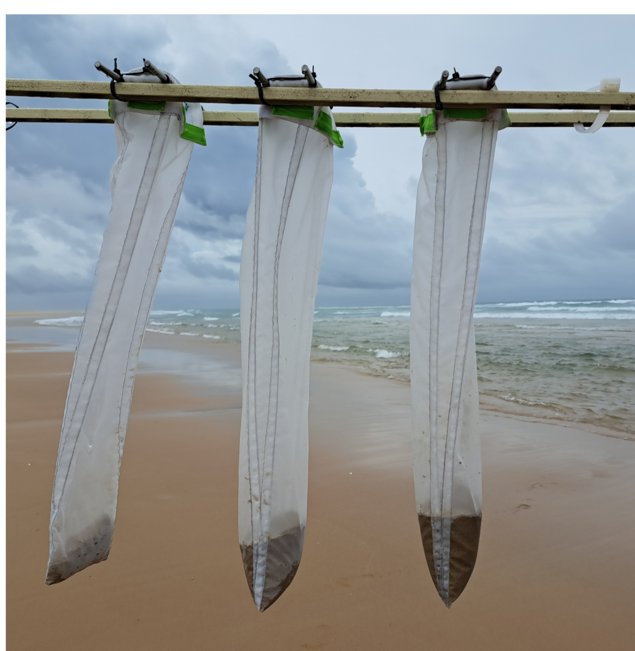
Figure 2. Low-cost sediment trap with three streamers placed at different depths
