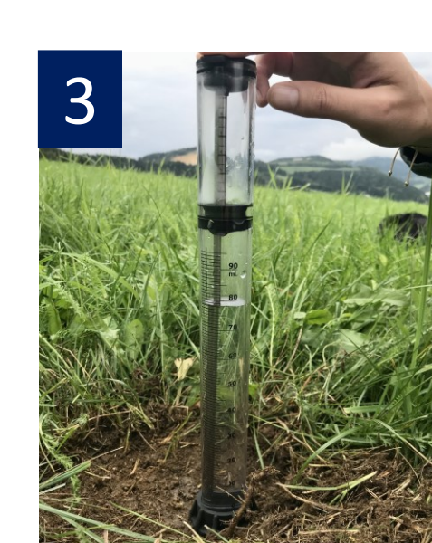
Figure 2: 1. ring for taking soil samples 2. Samples sieved and dried in the oven 3. Mini disc infiltrometer
