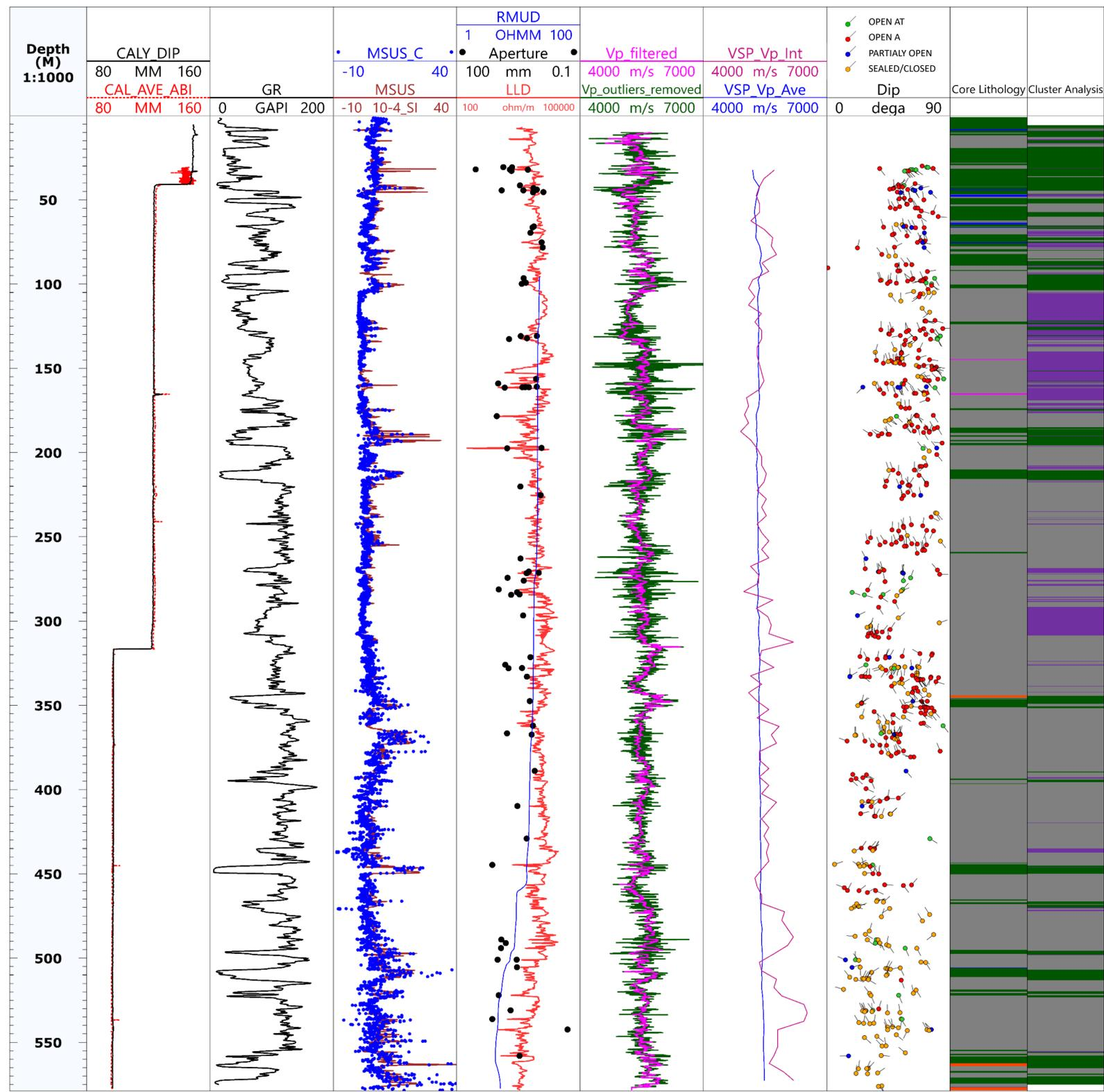
Figure 1: DT-1b borehole data: Caliper, Gamma ray (GR), wireline (MSUS) + core magnetic (MSUS\_C) susceptibility, deep electrical resistivity (LLD) + mud resistivity (RMUD) + aperture of open fractures, sonic P-wave velocity (Vp), VSP P-wave velocity, fracture dip, core lithology, cluster analysis
