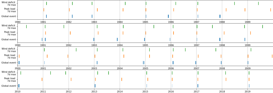
Figure: Extreme periods (for each year \max_t \sum_{i=0}^{168} dem_{t-i}^{eur} , \max_t \sum_{i=0}^{168} [dem_{t-i}^{eur} - gen_{t-i}^{onwind}] ) vs. our approach
